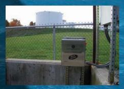
Slick Sleuth™ Oil Detection Systems are used for real-time detection of oil leaks and spills on fresh, brackish or saltwater and also on ground and other surfaces. The sensor is used to detect a wide range of oils and petroleum derivatives which include crude oil, fuel oil, lube oil, turbine oil, hydraulic oil, motor oil, gasoline and jet fuel, as well as various food oils, process oils and many others. Slick Sleuth is a UV-fluorosensor, using the same highly-sensitive optical method for sensing
